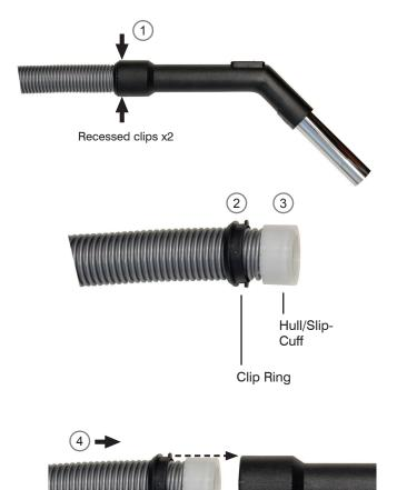
1. Remove the existing handle from your vacuum hose by detaching the clip ring at the rear of the handle.
